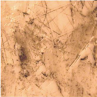
The partly micro-fine greases, residues and dust dirt even settles in the smallest capillary grooves and cannot be removed efficiently using standard cleaning tools like brushes or sponges.
